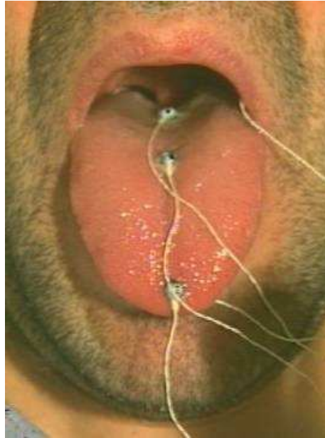
Figure 3.2-1. Picture of a subject's tongue with three EMA coils attached to the tongue
