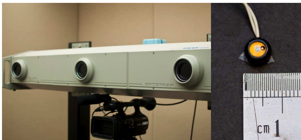
Figure 4.1. The OPTOTRAK infrared camera unit (left) tracks the three-dimensional position over time of infrared emitting markers, measuring 7mm in diameter (right) with high spatial and temporal resolutions.
