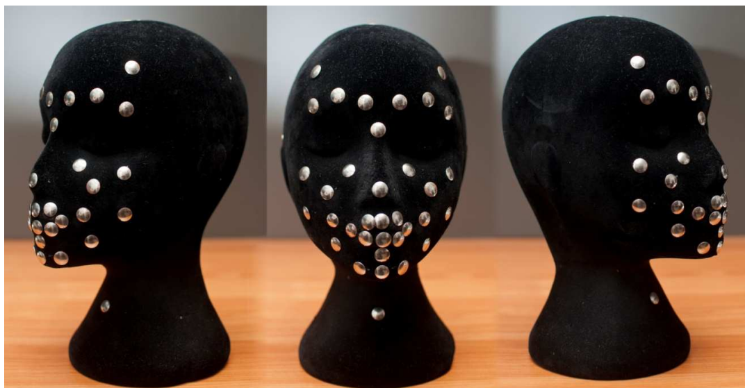
Figure 4.2. A polystyrene foam head was used as a visual guide to ensure that placement of the optical markers was consistent across talkers.
