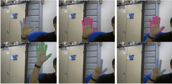
Fig. 5. Hand tracker with current posture and image motion (color) recognition: some snapshots from a tracking sequence
