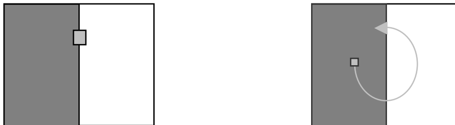
Figure 44: Stimulus presented on the screen during the synchronization procedure: left: initial image; right: indicated circular movement of gaze target to generate smooth a sequence of valid gaze data.
