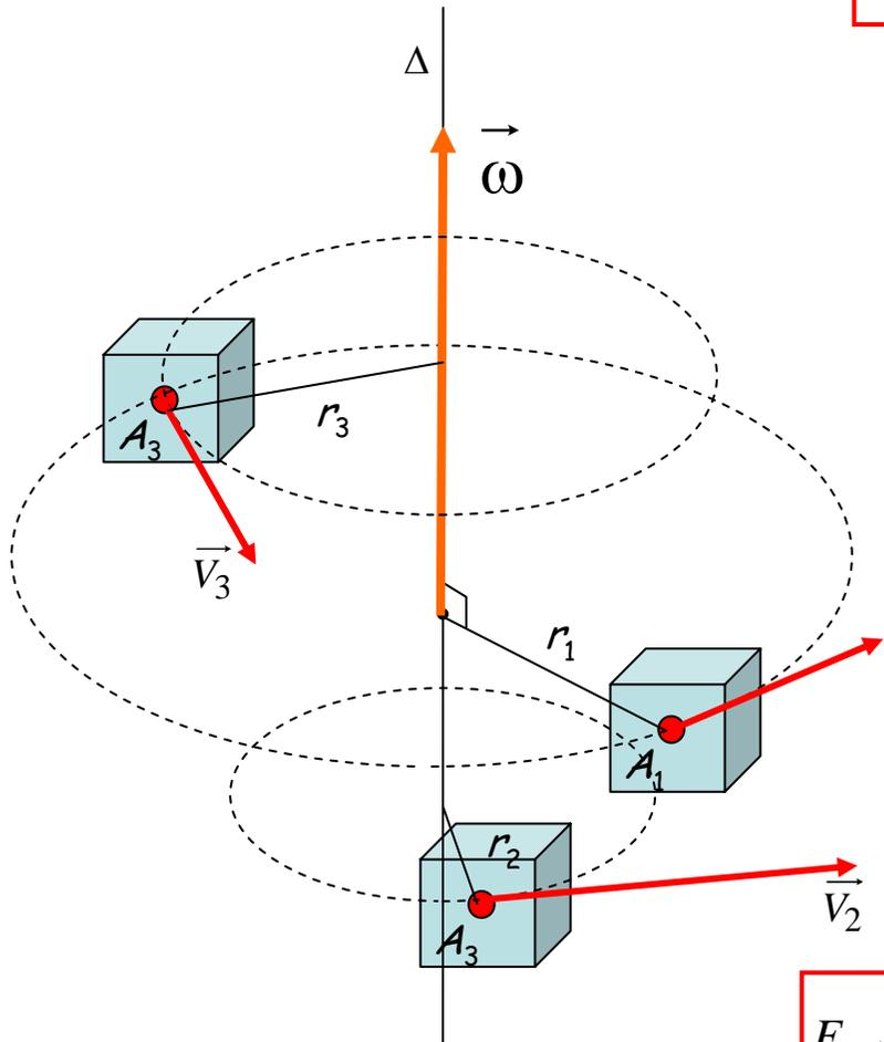
$$V_1 = r_1 \cdot \omega \quad \frac{1}{2} m_1 V_1^2 = \frac{1}{2} m_1 r_1^2 \omega^2$$
