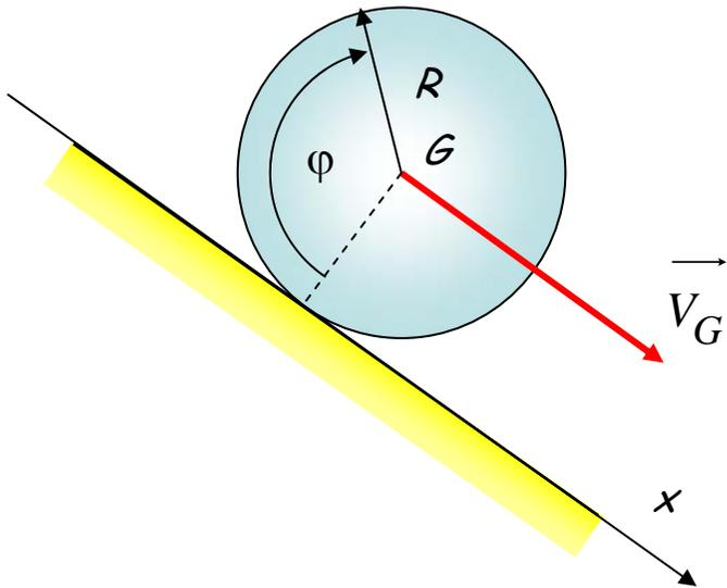
$$V_G = \frac{dx}{dt} = R \frac{d\varphi}{dt} = R\omega \quad \omega = \frac{V_G}{R}$$
