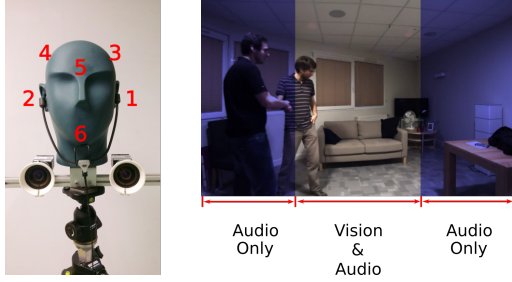
Fig. 2. (a) Robotic head with 6 microphones (red numbers); (b) Experimental simulation of limited field-of-view.
