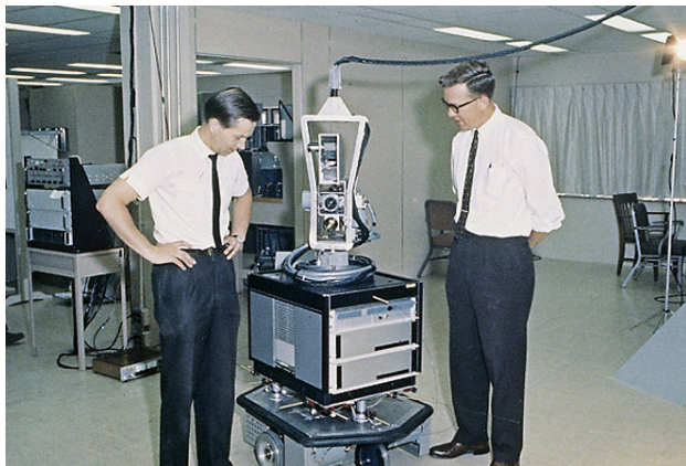
Shakey robot from Stanford Univ. Platform used to show first results on AI (1969)
