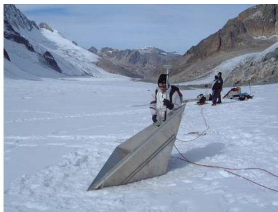
Figure 3 : Measurement of the position of a corner reflector by GPS (Argentière glacier).
