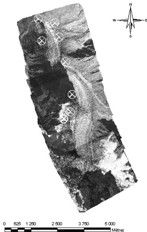
Figure 1. Set of the photos taken over the Mer de Glace in 1995. Circular marks represent the GCPs measured by GPS.
