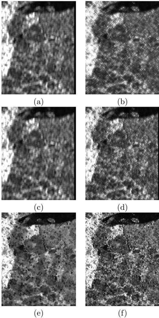
Figure 2:  $T_{11}$  intensity filtering results [ $171 \times 216$  pixels  $\mathbf{Z}_1$  of Fig. 1]: (a) BF, (b) BF-LLMMSE, (c) IDDN, (d) IDDN-LLMMSE, (e) IDAN, (f) IDAN-LLMMSE.
