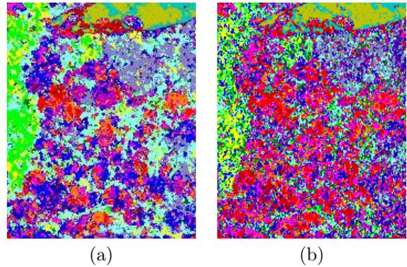
Figure 3: Wishart  $H - \alpha$  classification of the filtered  $T_{11}$  intensity image [ $171 \times 216$  pixels]: (a) using IDAN, (b) using IDAN-LLMMSE.
