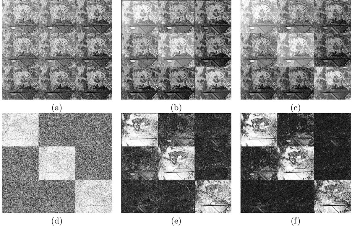
Figure 1: POL-InSAR data  $[4620 \times 4221 \times 3 \text{ pixels}]$ : (a) original master coherence, (b) BF filtered master coherence, (c) ADAN estimated master coherence, (d) original coherence map, (e) BF filtered coherence, (f) ADAN estimated coherence.
