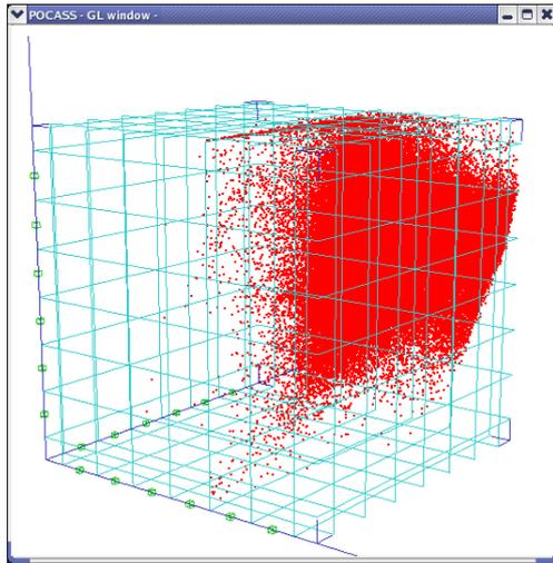
Figure 7. 3D histogram of the POL-InSAR attributes from Fig. 6. The mesh within the attribute space corresponds to the interactive tuning of the words used in the fuzzy fusion.
