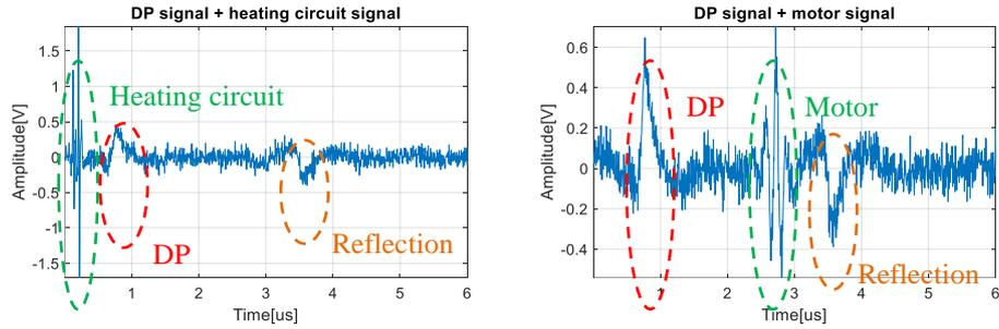
**Fig. 3.** The signal transmitted in the network in the presence of the DP signal and: heating circuit (left), motor (right)
