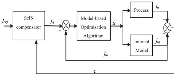
Fig. 1. MPC structure with self-compensator.
