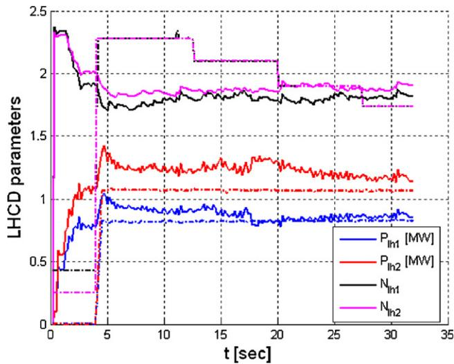
Fig. 2. LHCD parameters in closed loop (solid line) computed in simulation and experimental values (point-dashed) from pulse TS#35109.
