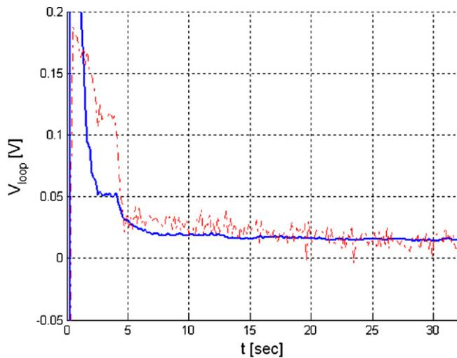
Fig. 3. Loop voltage in closed loop (solid) computed in simulation and experimental value (point-dashed) from pulse TS#35109.
