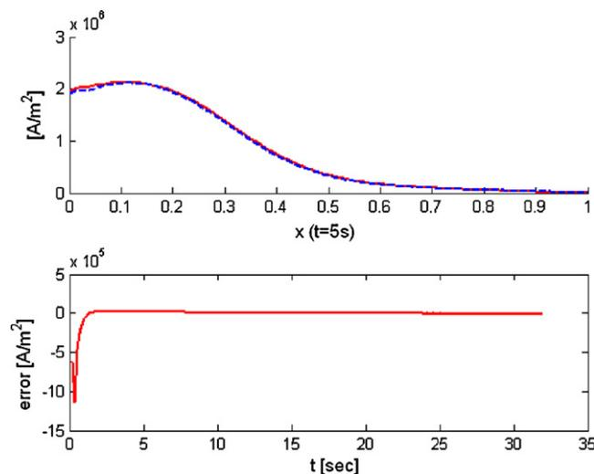
Fig. 4. (Top) Simulated plasma current profile in closed loop (solid) and desired value (dashed) at time  $t=5$  s. (Bottom) Mean control error.
