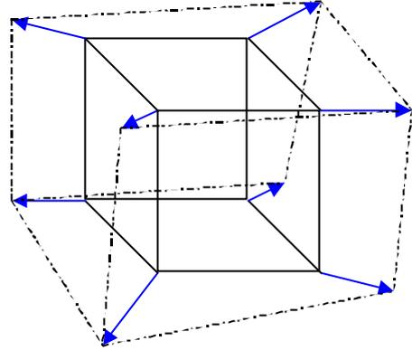
Figure 7: Applying a trilinear transformation to a cube.
