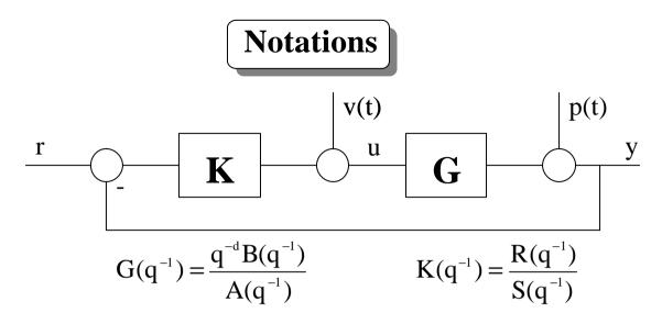
Sensitivity functions :  $S_{yp}(z^{-1}) = \frac{1}{1+KG}$ ;  $S_{up}(z^{-1}) = -\frac{K}{1+KG}$ ;  $S_{yv}(z^{-1}) = \frac{G}{1+KG}$ ;  $S_{yr}(z^{-1}) = \frac{KG}{1+KG}$ Closed loop poles :  $P(z^{-1}) = A(z^{-1})S(z^{-1}) + z^{-d}B(z^{-1})R(z^{-1})$
