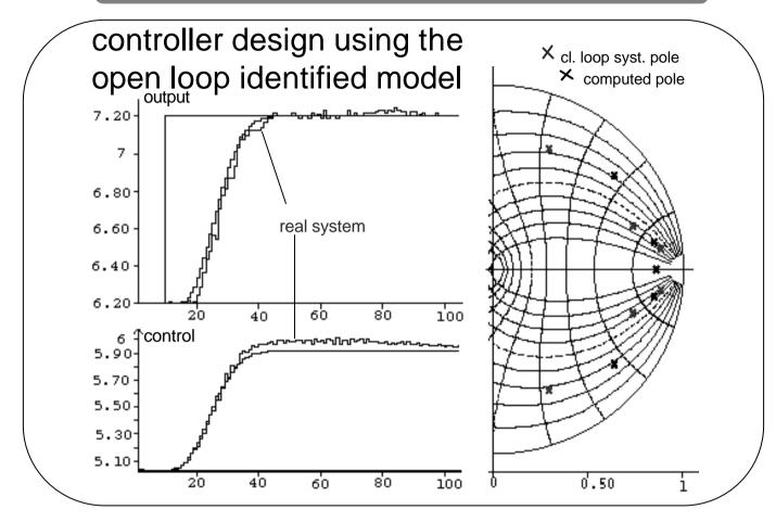
The pattern of *identified closed loop poles* is different from the pattern of *computed closed loop poles*
