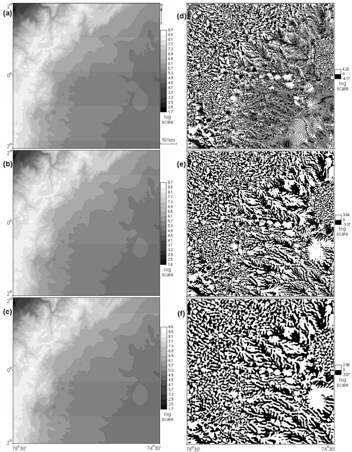
Fig. 3. DTM denoising. Elevation maps derived from the initial DEM (a), reconstructed from the ET 1-100 (b), and 1-50 (c);  $k_h$  maps derived from the initial DEM (d), the DEM reconstructed from the ET 1-100 (e), and 1-50 (f).
