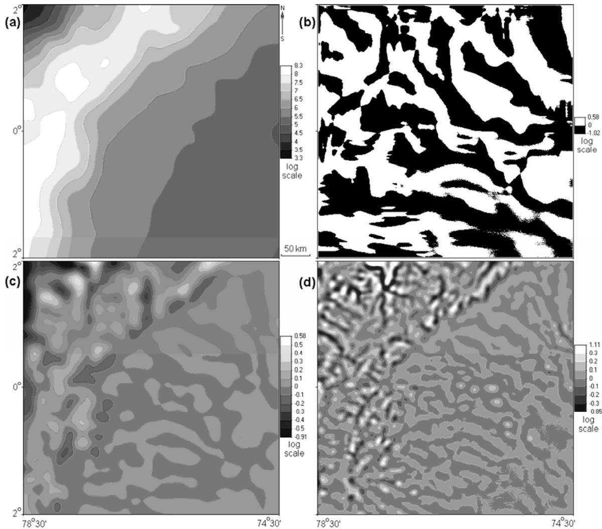
Fig. 4. Low-frequency components. Elevation maps reconstructed from the ET 1 (a), 2-3 (c), and 4-25 (d); (b)  $k_h$  map derived from the DEM reconstructed from the ET 1.
