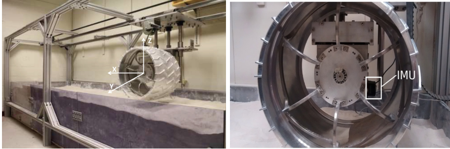
(a) MSL flight spare wheel in MIT's testbed (b) Position of the IMU sensor on the MSL wheel
