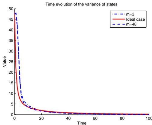
Fig. 5. Performance (variance of states) for the zooming in- zooming out method on a random geometric graph of 20 agents for different values of  $m$ . The convergence is almost not dependent on  $m$ .  $k_{in} = 0.8$ ,  $k_{out} = 2$ .
