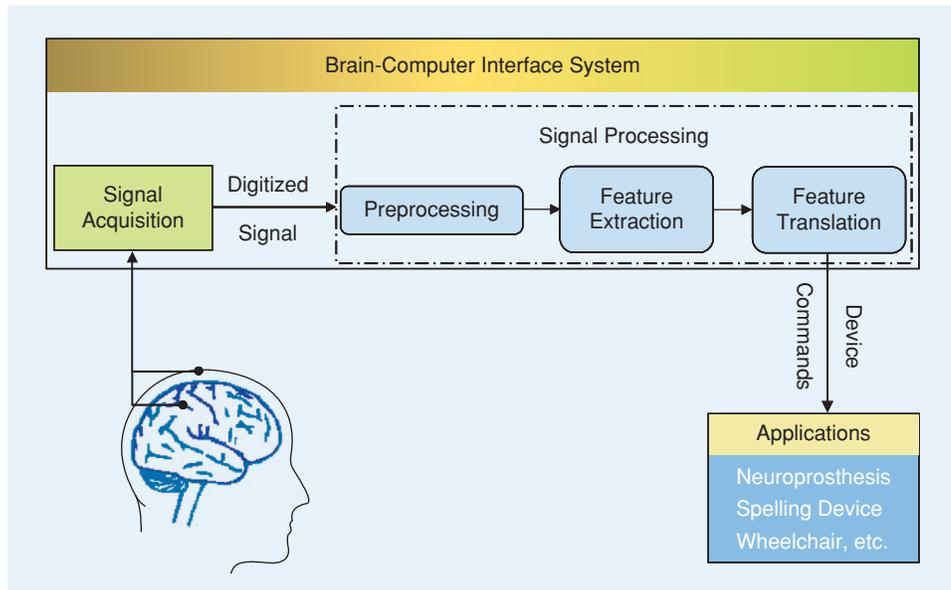
**[FIG1] Basic design and operation of any BCI system.**
