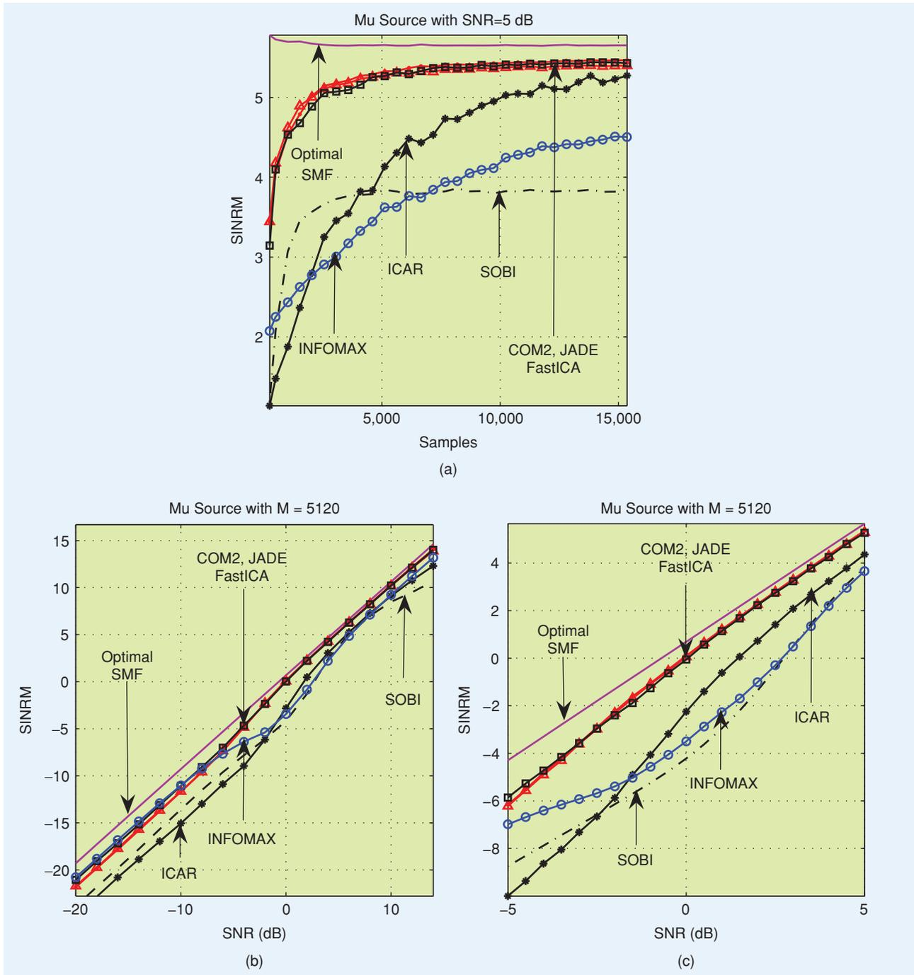
**[FIG3]** Evolution (in dB) of SINRM of sources as: (a) a function of data length with a SNR equal to 5 dB (b) as a function of SNR. (c) Represents the zoom in (b) for SNR between -5 dB and 5 dB.
