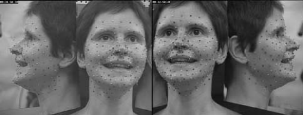
Figure 2: Gathering fleshpoint positions using a photogrammetric method. Here 245 colored beads have been glued on the subject's face.
