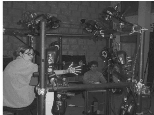
(b) Experimental setting for capturing the hand motion in free space
