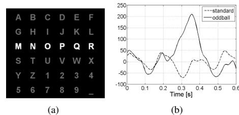
Fig. 1. Brain-Computer Interface "P300 speller". Fig. 1(a): screen display as was shown to the subjects with an highlighted row. Fig. 1(b): time course of the actual average signal waveforms at  $C_z$ .
