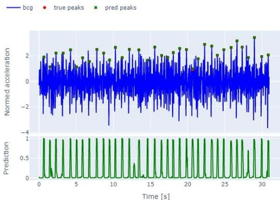
Figure 8. Example of BCG signal (blue line) with the U-Net output IJK prediction probability (green line), the true J peaks (red dot) and the heartbeat detection algorithm predicted J peaks (green cross).
