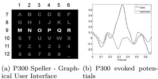
**Figure 1. P300-BCI Speller. Fig. 1: screen display, Fig. 1(b): average P300 response on one sensor located on Cz**
