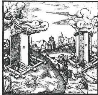
A—SILLS, B—POINTED STAKES, C—CROSSBEAMS, D—UPRIGHT PLANKS, E—RISERS, F—WINDS, G—COVERING, H—SCRAPE, I—MACHINE WITHOUT A COVERING
