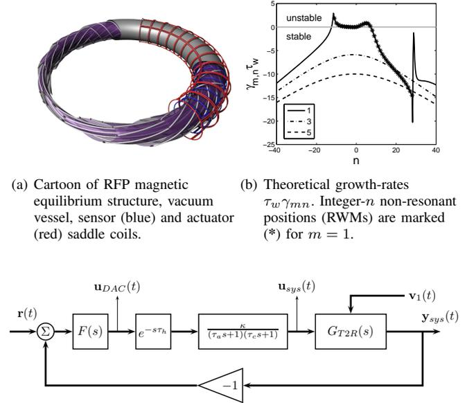
(c) Closed-loop schematics. Taps indicate available measurements.
