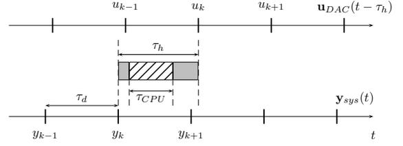
Fig. 2. Delay from control system. Note  $\tau_h$ , dependent of control algorithm, possibly greater than  $\tau_d$  but obviously  $\tau_{CPU} < \tau_d$  for a working system. Sample frequency  $f_s = 1/\tau_d$ . Input  $y_k$  sampled from sensor coils, output  $u_k$  is the DAC-output subsequently fed to the active coil amplifiers as augmented system input.
