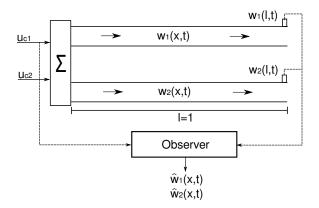
Fig. 1. Schematic of the estimation problem
