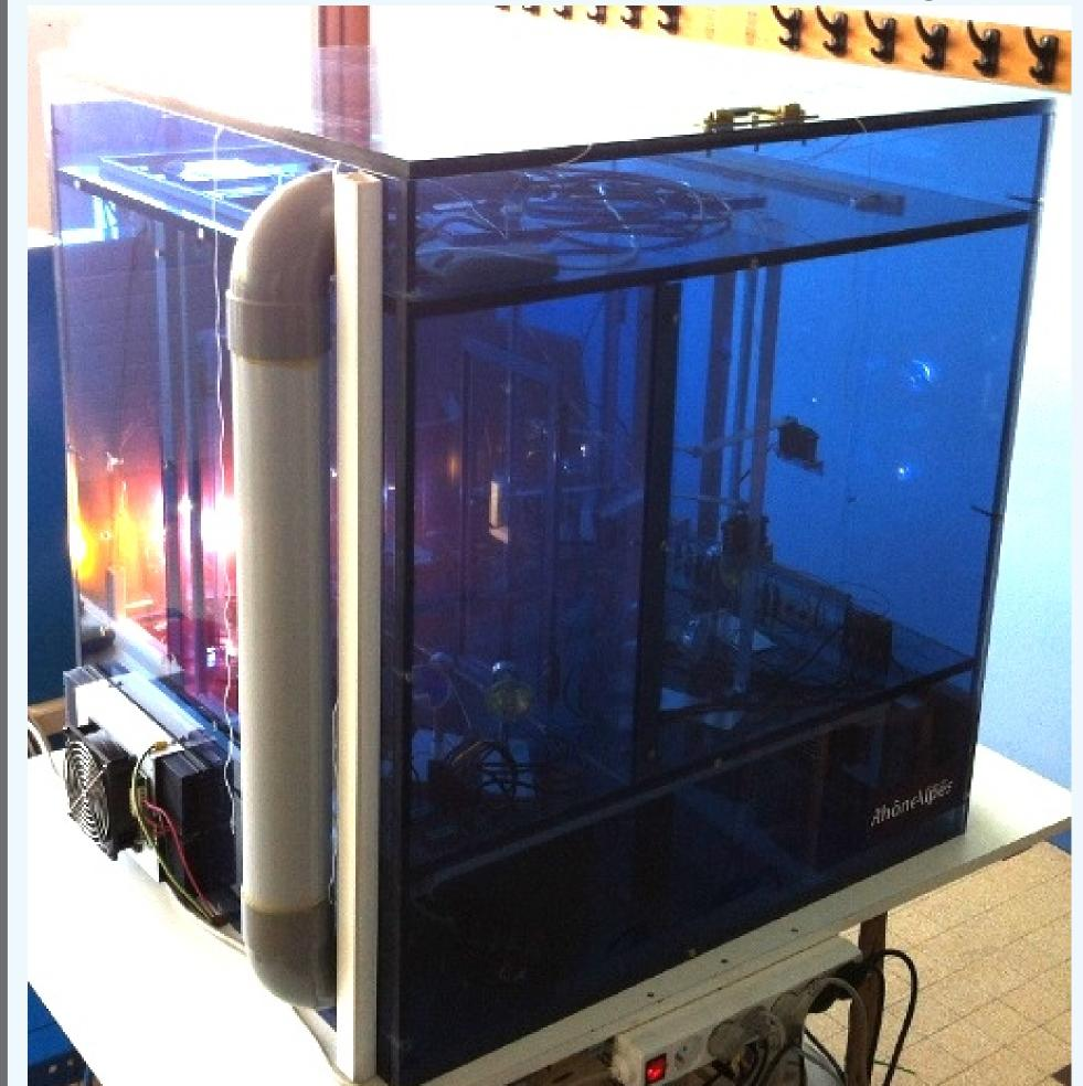
This small-scale experiment of a flat equipped with *UnderFloor Air Distribution* is built at the physics department (UFR PhITEM) of University Joseph Fourier, Grenoble, France.
