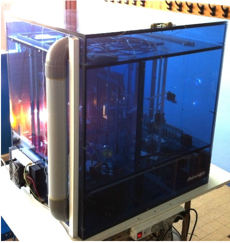
Fig. 2. Small-scale experiment of a flat with UFAD regulation 2
