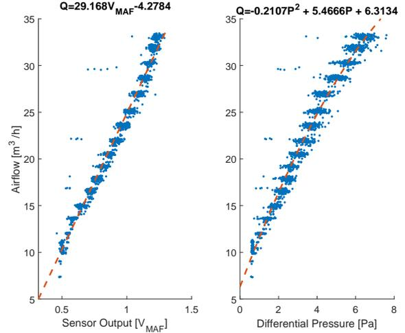
Figure 7. Calibration of the mass air flow sensor (left) and of the orifice plate sensor (right) using the hot wire measurement and a curve fitting method.
