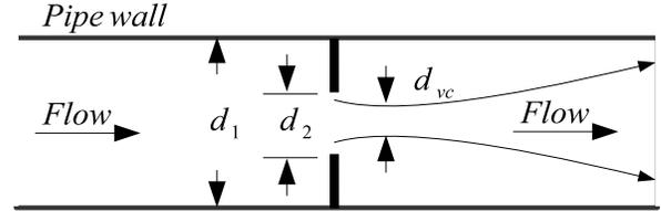
Figure 4. Schematic view of an orifice plate sensor.
