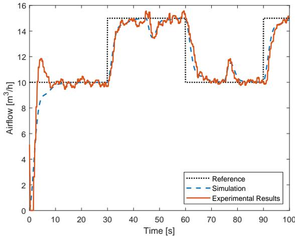
Figure 9. Controlled response of the airflow in the ventilation network.
