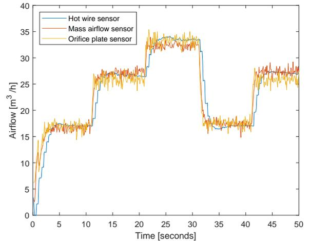
Figure 8. Comparison of the air flow measurements for the three sensors.
