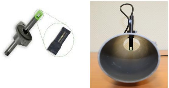
Figure 2. EE671 hot wire sensor connected to a pipe.
