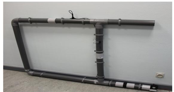
Figure 5. Benchmark: A ventilation network configuration.
