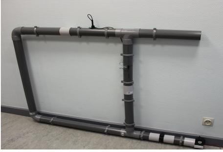
**FIGURE 2** Experimental benchmark for underground mining ventilation network.
