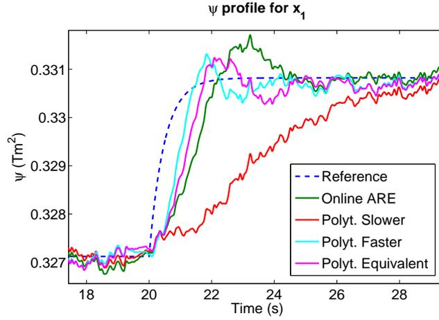
Figure 4. Regulation around  $\bar{\psi}$  for  $\psi_1$  with the LPV approach. The thin dashed line is the reference, the solid line is the ARE-based simulation (first approach) and the others are polytopic (LPV) regulators with different  $\gamma$  values.
