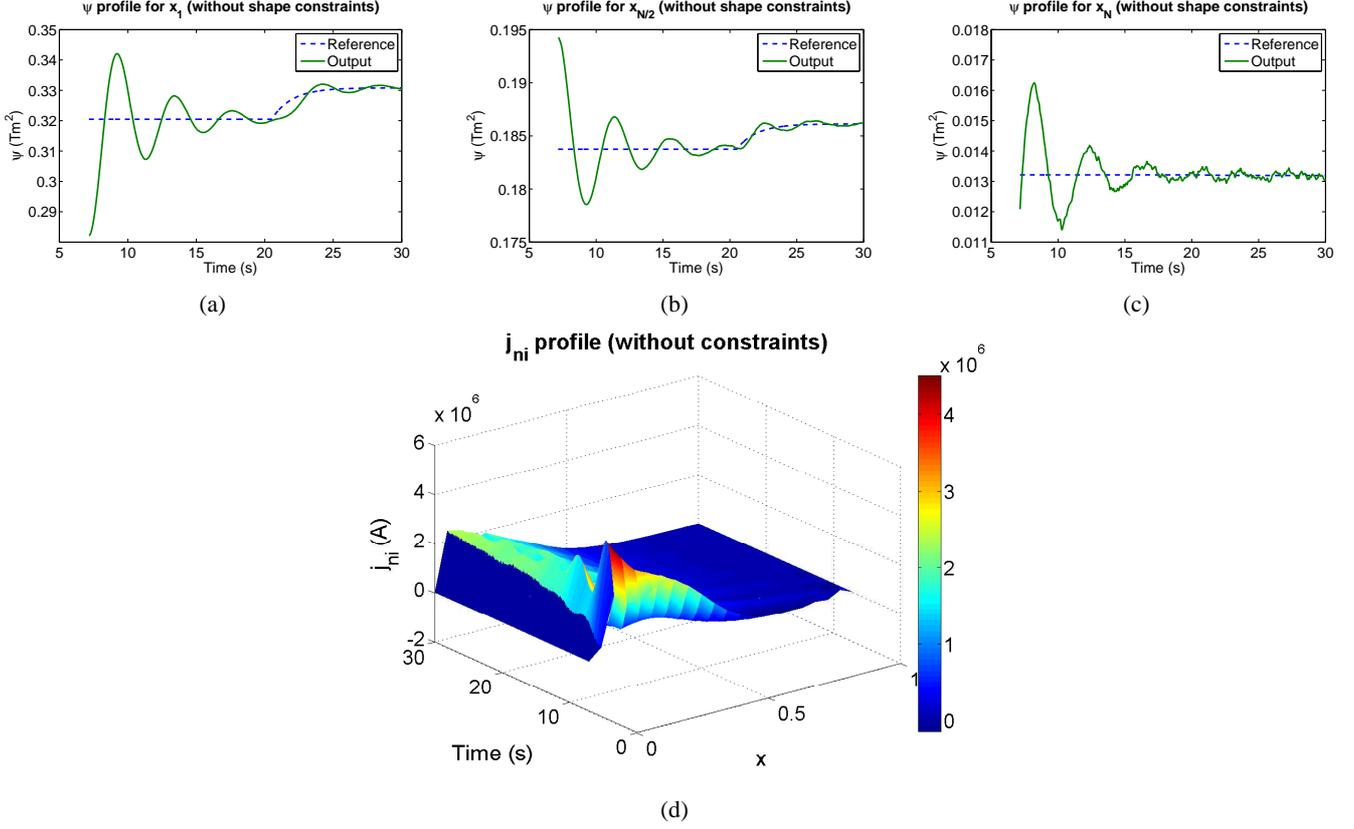
Figure 1. Regulation around  $\bar{\psi}$  with the unconstrained controller (plain line: numerical simulation, dashed line: the reference). (a) Evolution and reference of the state  $\psi_1$  (plasma center); (b) evolution and reference of the state  $\psi_{N/2}$  (mid radius  $a/2$ ); (c) evolution and reference of the state  $\psi_N$  (plasma edge); (d) applied control signal  $u$ .
