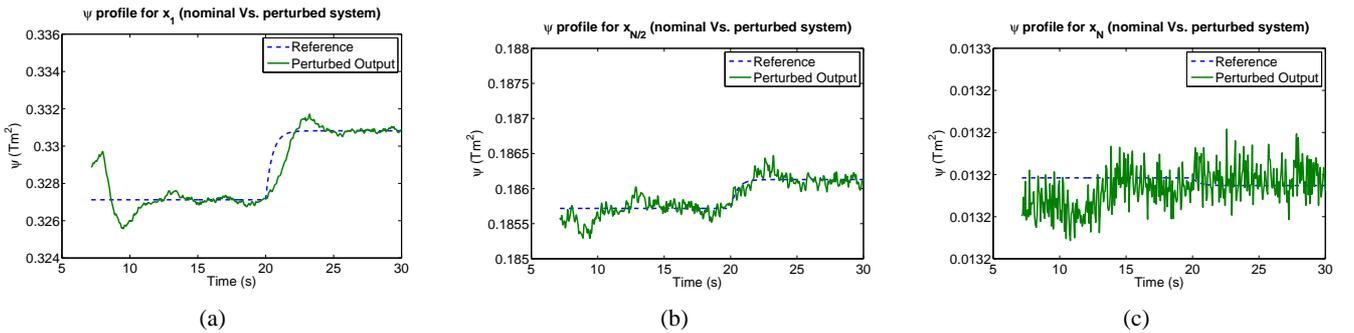
Figure 3. Reference and perturbed output caused by an error in the estimation of  $\eta_{\parallel}$  (dashed line: reference, solid line: numerical simulation).
