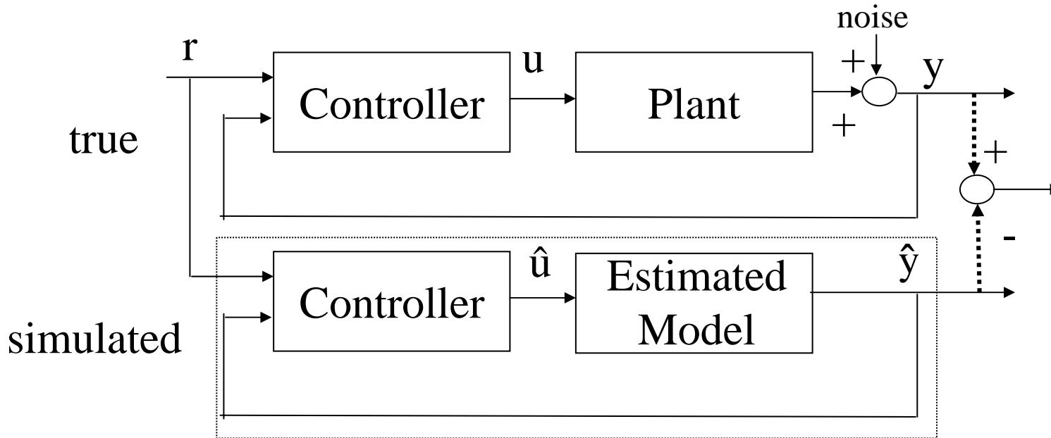
If the estimated model is good, the poles of the « true » loop and of the « simulated » loop should be *close*
