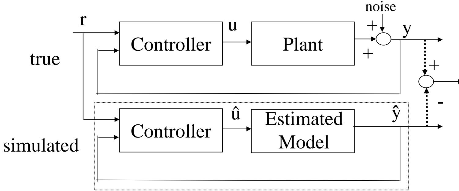
If the estimated model is good, the sensitivity functions of the « true » loop and of the « simulated » loop should be *close*
