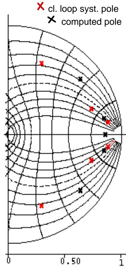
The pattern of *identified closed loop poles* is different from the pattern of *computed closed loop poles*
