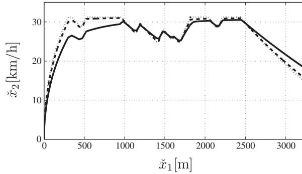
Figure 23. Dotted line, reference  $\check{x}_2^*$ ; dashed line, tracking response of the nonlinear system with a mass variation of 10%; solid line, tracking response of the nonlinear system with a mass variation of 50%.
