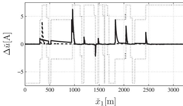
Figure 25. Dotted lines,  $\Delta u_{min}(k)$  and  $\Delta u_{max}(k)$ ; dashed line, tracking input  $\Delta\check{u}(k)$  of the nonlinear system with a mass variation of 10%; solid line, tracking input  $\Delta\check{u}(k)$  of the nonlinear system with a mass variation of 50%.
