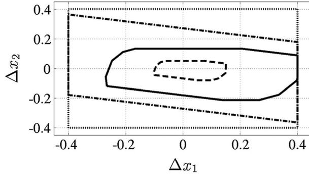
Figure 8. Dotted line, constraint  $X_{\Delta}(k)$ ; dash-dotted line, constraint  $\mathcal{X}_{\Delta}(k)$ ; dashed line, nominal invariant set  $\hat{\Omega}$ ; solid line,  $\alpha(k)\hat{\Omega}$  with  $\alpha(k) = 2.67$ .
