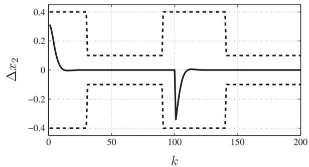
Figure 15. Solid line, tracking error and  $\Delta x_2(k)$ ; dashed line, time-varying constraints.
