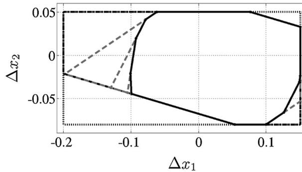
Figure 2. Grey dashed lines, pre-images of  $\mathcal{X}_{\Delta}$ ; solid line, final invariant set  $\Omega$ .
