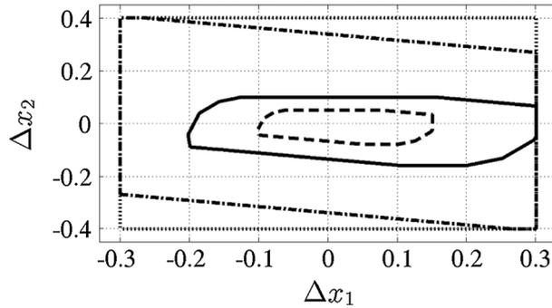
Figure 10. Dotted line, constraint  $X_{\Delta}(k)$ ; dash-dotted line, constraint  $\mathcal{X}_{\Delta}(k)$ ; dashed line, nominal invariant set  $\hat{\Omega}$ ; solid line,  $\alpha(k)\hat{\Omega}$  with  $\alpha(k) = 2$ .
