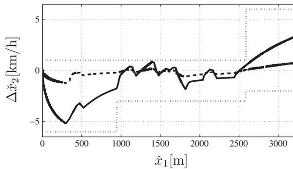
Figure 24. Dotted lines,  $\Delta x_{2min}(k)$  and  $\Delta x_{2max}(k)$ ; dashed line, tracking error  $\Delta\check{x}_2(k)$  of the nonlinear system with a mass variation of 10%; solid line, tracking error  $\Delta\check{x}_2(k)$  of the nonlinear system with a mass variation of 50%.
