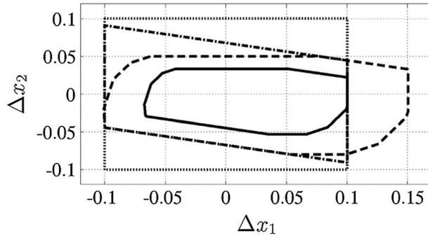
Figure 9. Dotted line, constraint  $X_{\Delta}(k)$ ; dash-dotted line, constraint  $\mathcal{X}_{\Delta}(k)$ ; dashed line, nominal invariant set  $\hat{\Omega}$ ; solid line,  $\alpha(k)\hat{\Omega}$  with  $\alpha(k) = 0.67$ .
