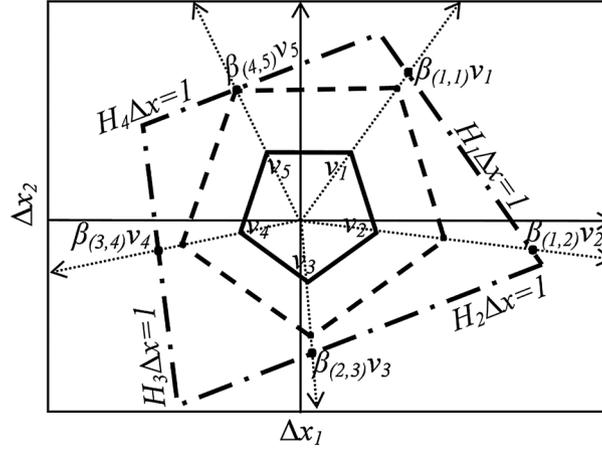
Figure 3. Solid line, polytopic invariant set  $\hat{\Omega}$ ; dashed line, homothetic copy of  $\hat{\Omega}$  at time  $k$ ; dash-dotted line, polytopic constraints  $\mathcal{X}_\Delta$  at time  $k$ ;  $\beta_{(i,j)}v_j$ , homothetic vector of  $v_j$  (along the dotted vectors) with factor  $\beta_{(i,j)}$  at time  $k$  (time index  $k$  not reported).
