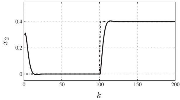
Figure 13. Solid line, tracking response of  $x_2(k)$ ; dash-dotted line, reference.
