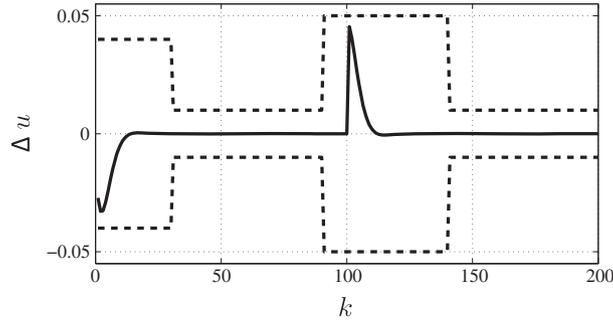
Figure 16. Solid line, tracking error  $\Delta u(k)$ ; dashed line, time-varying constraints.
