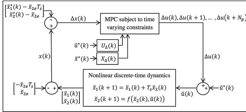
Figure 21. Closed-loop implementation of the time-varying MPC. The function that describes the velocity  $\dot{x}_2(k+1) = f(\dot{x}_2(k), \ddot{u}(k))$  is given by (44).
