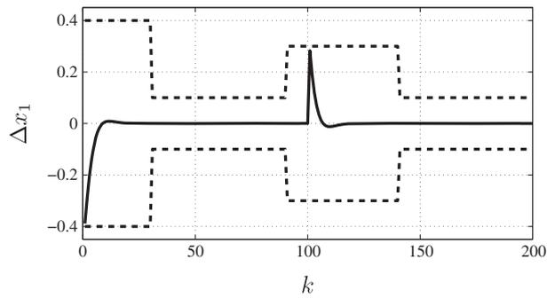
Figure 14. Solid line, tracking error  $\Delta x_1(k)$ ; dashed line, time-varying constraints.
