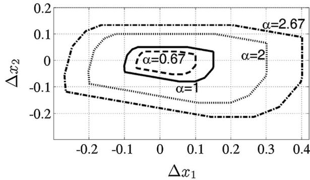
Figure 11. Solid line, nominal invariant set  $\hat{\Omega}$ ; dashed line,  $0.67\hat{\Omega}$ ; dotted line,  $2\hat{\Omega}$ ; dash-dotted line,  $2.67\hat{\Omega}$ .
