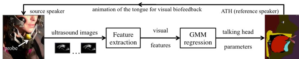
Figure 1. Proposed system of visual feedback based on the automatic animation of an articulatory talking head from ultrasound imaging.
