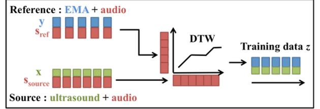
Figure 2. Time-alignment of ultrasound/EMA articulatory data of the tongue recorded on the source/reference speaker using DTW
